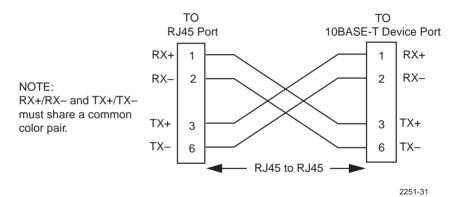
Figure 3-8 Cable Pinouts - RJ45 Crossover Cable
